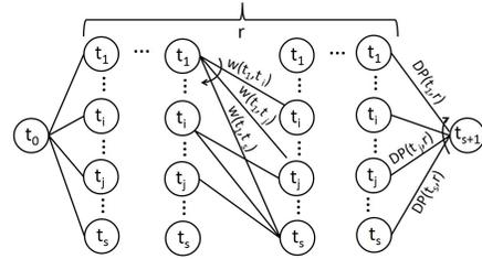
Figure 5: Dynamic programming approach of 2D-RRMS Algorithm.
